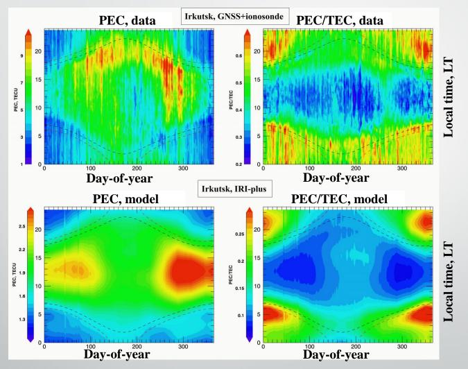
The local time versus day-of-year distributions of PEC (left) and PEC/TEC ratio (right) from experimental data (top) and the IRI-Plas model simulations (bottom). PEC and PEC/TEC ratio distributions feature significant diurnal and seasonal variations.
