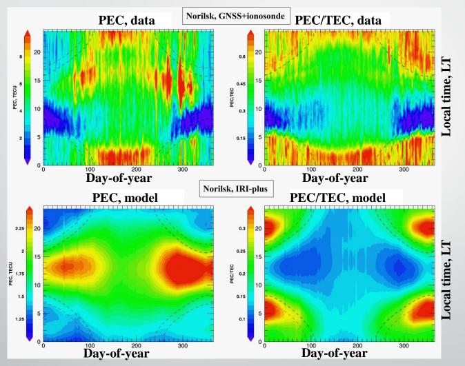
The same distributions for Norilsk. The model underestimates the level of the plasmasphere contribution. But general dynamics from experimental data and IRI-Plas model are close.
