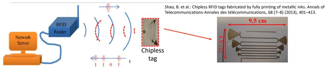
Information is encoded by connecting the antenna to a passive network with discontinuities that generate delayed echoes of the incoming signal.
