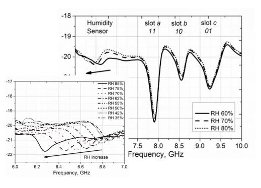
Resonator coated with a humidity sensitive material
