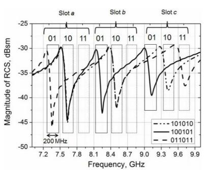
The ID of the tag is encoded by a spectral signature. The presence or the lack of a resonance corresponds to a 1 or 0 bit. Typically, the ID cannot be re-writeable because it is included in the structure of the tag, nevertheless there are example in the literature showing investigations to make chipless tag re-writable.
