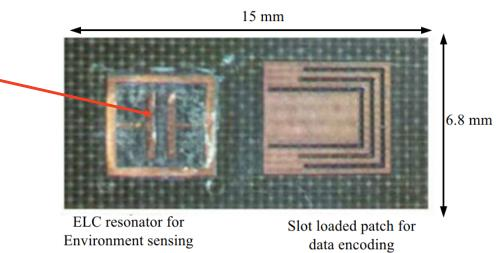
The mechanism for sensing is based on frequency shifts.
