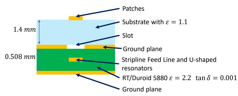
$(60 \times 20 \times 2) mm^3$  dielectric layers and ground plane are hidden
