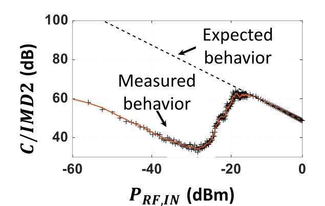
High IMD2 for  $P_{RF,IN} \in [-60, -24]dBm \rightarrow$  Cause: Rayleigh Backscattering
