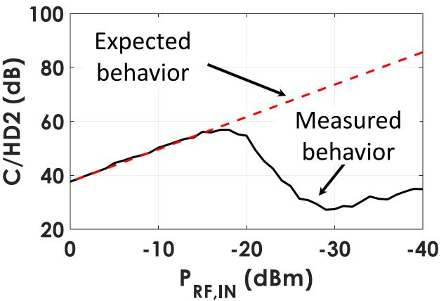
High HD2 for  $P_{RF,IN} \in [-60, -24]dBm \rightarrow$  Cause: Rayleigh Backscattering
