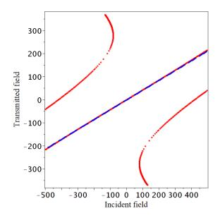
Puc. .5: Amplitude of the transmitted field  $F_T$  vs amplitude of the incident field  $F_I$  in the linear ( $\alpha = 0$ , blue) and nonlinear (red) cases. The values of parameters are $\gamma = 1.15$ ,  $k_0^2 = 1$ ,  $r_0 = 2$ , r = 4,  $\varepsilon^2 = 4$ ,  $\alpha = 10^{-3}$ .
