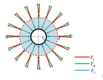
**Puc.** 1: Waveguide  $\Sigma$ , where  $r_0$  and r are the radii of the internal (perfectly conducting) and external (dielectric) cylinders, respectively.
