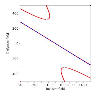
Puc. .4: Amplitude of the reflected field  $F_R$  vs amplitude of the incident field  $F_I$  in the linear ( $\alpha = 0$ , blue) and nonlinear (red) cases. The values of parameters are $\gamma = 1.15$ ,  $k_0^2 = 1$ ,  $r_0 = 2$ , r = 4,  $\varepsilon^2 = 4$ ,  $\alpha = 10^{-3}$ .
