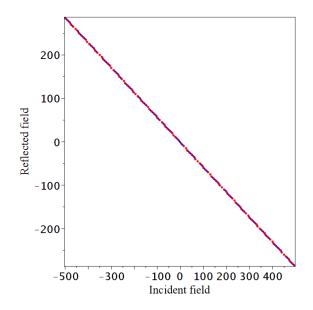
Puc. .2: Amplitude of the reflected field  $F_R$  vs amplitude of the incident field  $F_I$  in the linear ( $\alpha = 0$ , blue) and nonlinear (red) cases. The values of parameters are  $\gamma = 1.15$ ,  $k_0^2 = 1$ ,  $r_0 = 2$ , r = 4,  $\varepsilon^2 = 4$ ,  $\alpha = 10^{-5}$ .
