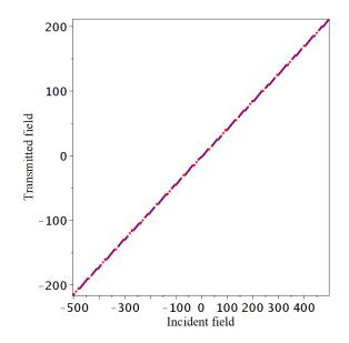
Puc. .3: Amplitude of the transmitted field  $F_T$  vs amplitude of the incident field  $F_I$  in the linear ( $\alpha = 0$ , blue) and nonlinear (red) cases. The values of parameters are  $\gamma = 1.15$ ,  $k_0^2 = 1$ ,  $r_0 = 2$ , r = 4,  $\varepsilon^2 = 4$ ,  $\alpha = 10^{-5}$ .
