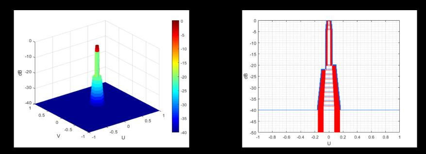
The layout of the used mask for beam forming, (left) 3D schematic view, (right) 2D schematic view showing the high mask (the blue one) and low mask (the red one).
