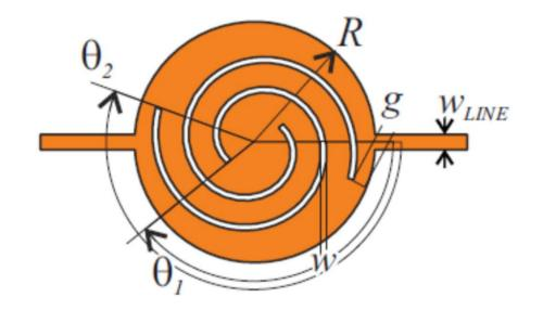
The filter geometry is shown here. The inner Archimedean spiral is defined by
