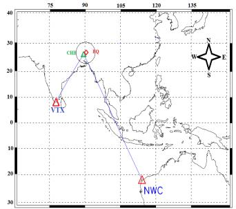
VLF radio ignal Receiving station, VLF transmitters with Great Circle Paths, EQ epicenter and the EQ preparation zone (circle)on global map. The blue lines are the VTX-CHB and NWC-CHB propagation paths.
