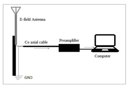
Schematic diagram of the VLF signal receiving system.
