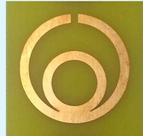
Figure 1. (a) Structure of a unit cell with its dimensions and field vectors ( r_1=12 mm, g=2 mm, t=2 mm, outer radius of the inner ring is 7 mm and center to center distance= 3.15 mm, a=30 mm) in FR4 substrate (b) Fabricated unit cell on FR4 substrate
