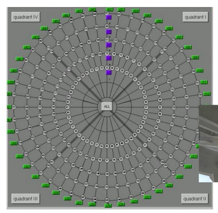
**248 panels** in six separate rings (innermost two are fixed).
