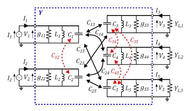
The entire multiport system (indicated by the dashed rectangle) is fully determined by the admittance matrix Y which is, at the resonance angular frequency  $\omega_0$ , equal to:
