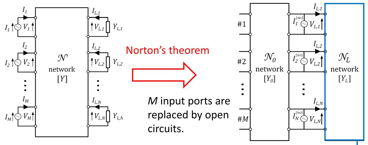
The *N* loads of the receiver are represented by the network  $\mathcal{N}_{L}$  described by the admittance matrix  $Y_{L}$ .
