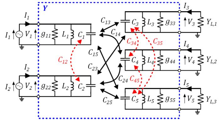
In order to obtain a resonant scheme, the inductors  $L_j$  are added:  $L_j = \frac{1}{\omega_0^2 C_j}$
