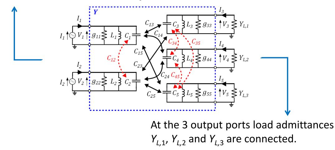
The shunt conductances  $g_{ii}$  (*j*=1,...,5) describe the losses in the circuit.
