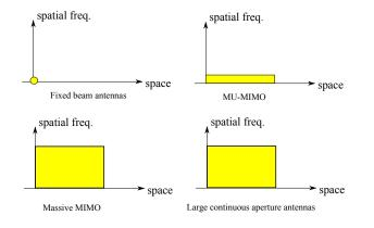
Different "kind of antennas" use different space/spatial bandwidth For example, Massive MIMO use a larger spatial bandwidth compared to standard MU-MIMO
