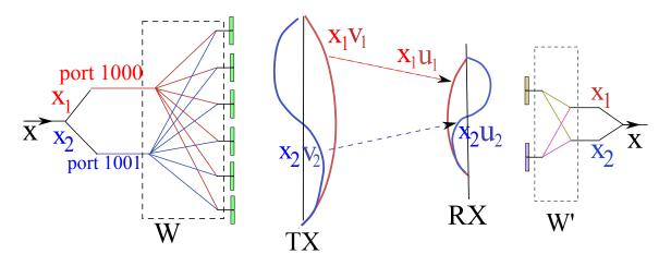
In case of planar radiating surfaces the SNDF is almost equal to 4 times to the electrical area of the radiating surface, i.e.  $4 \text{ A}/\lambda^2$ , wherein A is the area and  $\lambda$  is the wavelength The SNDF is the least upper bound for the number of spatial parallel channels (layers) of any communication system based on space coding
