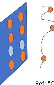
The density of the antenna elements must be higher in the area where the field has faster spatial variations [See Ref] We need the equivalent to a non uniform sampling of a (spatial) function whose local (spatial) bandwidth is not constant
