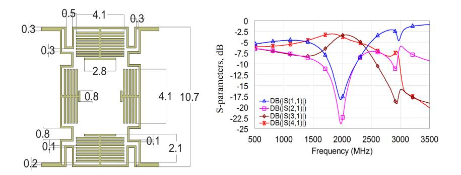
Fig. 3. Compact coupler design and characteristics .
