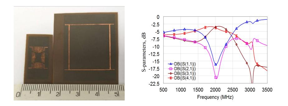
Fig. 6. Compact coupler design and characteristics .
