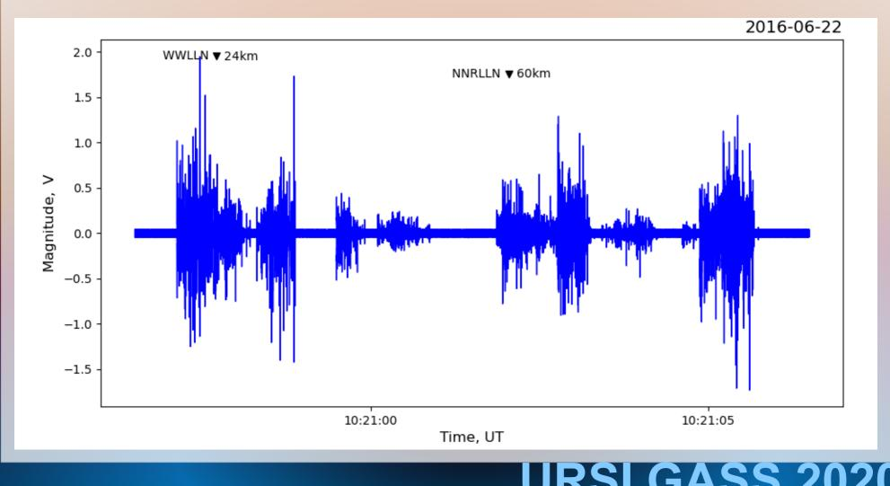
Another 10-second interval of confirmed continuity part at the middle part of the record — thunderstorm recession. Intervals of radio emission are separated by longer quiet ones. Registered by lightning location networks events are shown for distances up to 60 km.
