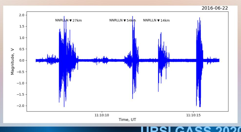
Other 10-second interval of confirmed continuity part at the middle part of the record — further thunderstorm recession. Registered by lightning location networks events are accompanied by radio emission. But some of the intervals of radio emission are not connected with such events.
