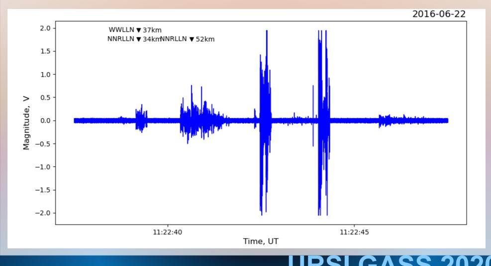
Scans of the radio emission at the beginning of an emission interval with different temporal resolution. Pulsed structure is clearly seen.
