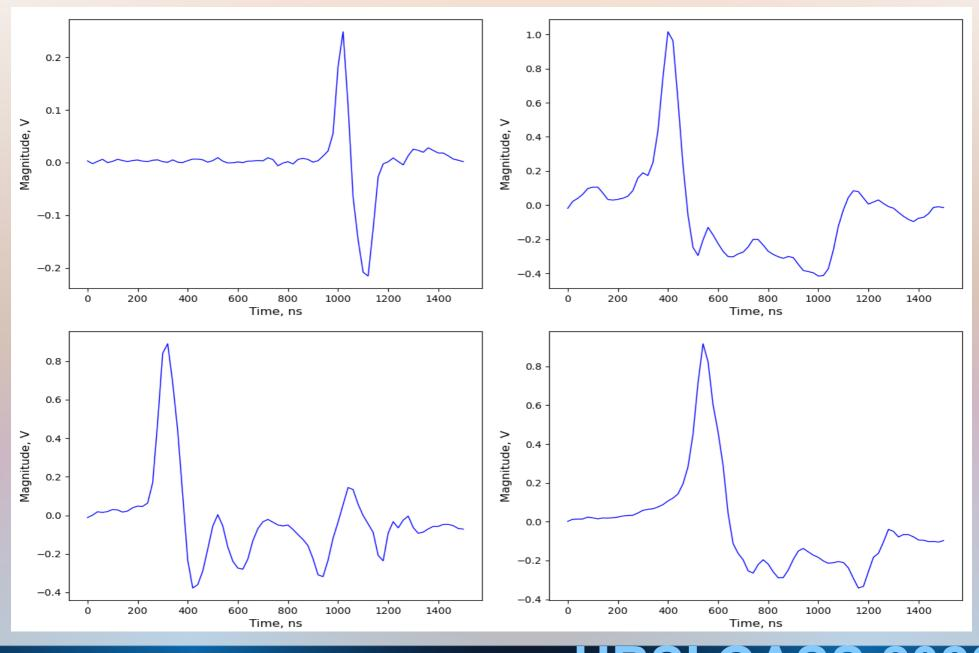
Comparison of the observed radio pulse form (solid) with the theoretical predictions of radio emission from runaway breakdown process initiated by an extensive atmospheric shower calculated in [A.V. Gurevich et.al., 2004, Phys. Lett. A 325, 389] (dash-dot) and [J.R. Dwyer, M.A. Uman, H.K. Rassoul, 2009, J. Geophys.Res., 114, 6867] (dash). *Borrowed from A.V. Gurevich, A.N. Karashtin, Phys. Rev. Lett., 2013, 110, 185005*
