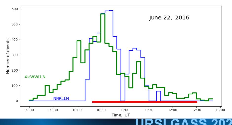
Radio frequency emission record started at 10:20:43 UT (LT  $\approx$  UT+3h). Root mean square over 1 millisecond intervals is shown. Record length 2<sup>h</sup> 9<sup>m</sup> 46<sup>s</sup>, data loss 4<sup>m</sup> 53<sup>s</sup> (~3.76%). 10:46-10:51 — switch off matching amplifier power to ensure that signal comes from antenna. Crosstalk on the cable is below the signal level from the antenna by at least 40 dB.
