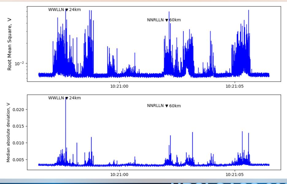
RMS/MAD and kurtosis values for the first shown above 10-second sample of radio emission from the thundercloud. Primarily pulsed nature of the emission is testified by both indicators.
