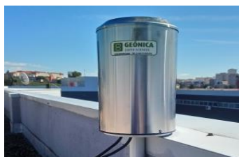
Weighing Rain Gauge (from 2017- nowadays)
