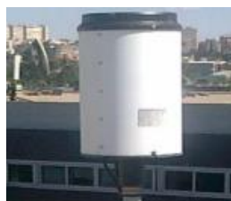
Tipping-Bucket Rain Gauge (untill Nov. 2017)
