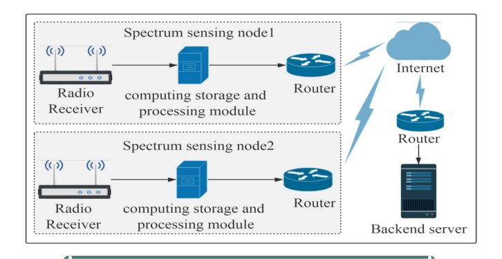
**Radio receiver** is used to collect the FM broadcast spectrum within the monitoring range.
