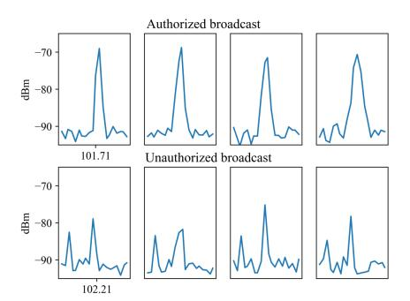
The peak value of the authorized broadcast channel is about - 70dBm, the shape of which is high and straight; the peak value of the unauthorized broadcast channel is about - 80dBm, the shape of which is short and often accompanied by side lobes.
