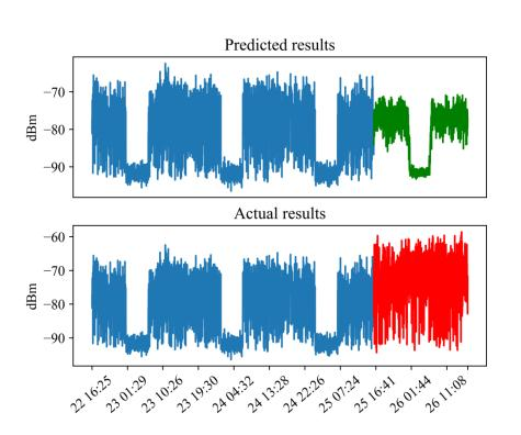
Predict the data of the fourth day through ARIMA model. The figure shows a comparison of the predicted data(the green line) and actual data(red line) of the fourth day. The predicted spectrum reveal that the frequency band is free at 1am on January 26, while the actual spectrum show that the frequency band is occupied.
