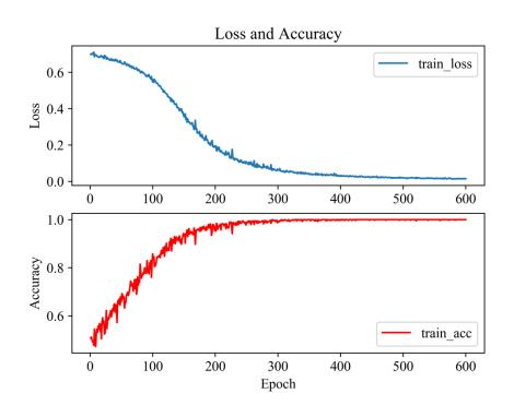
The training set of the neural network contains 1000 groups of broadcast spectrum data, and takes the spectrum peak of each channel as the characteristic training. The loss function converges to 0 at 600 epochs, and the accuracy is close to 1.
