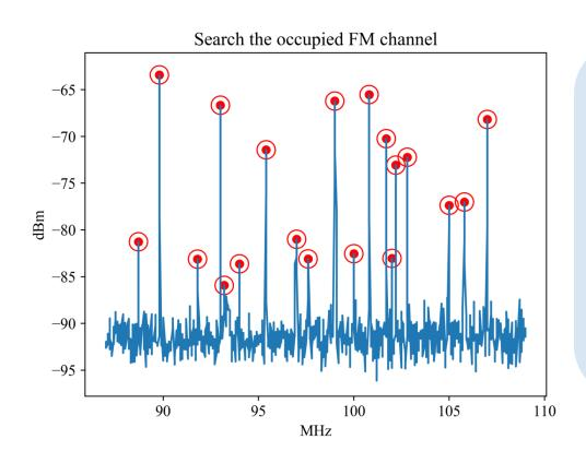
The FM frequency band is divided into 210 channels of which the bandwidth is 120kHz.
