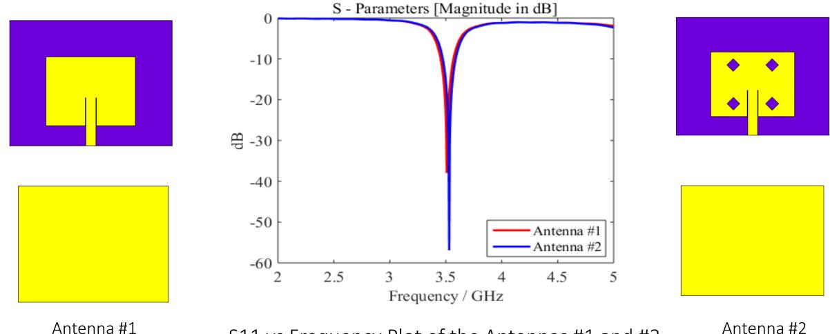
S11 vs Frequency Plot of the Antennas #1 and #2
