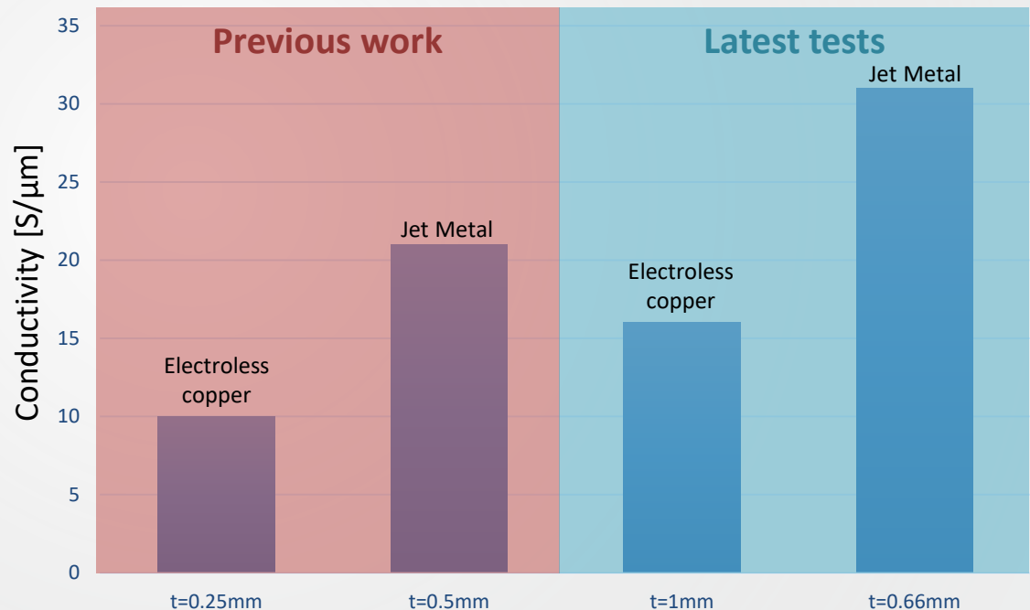
Metallization tests in Alumina substrates
