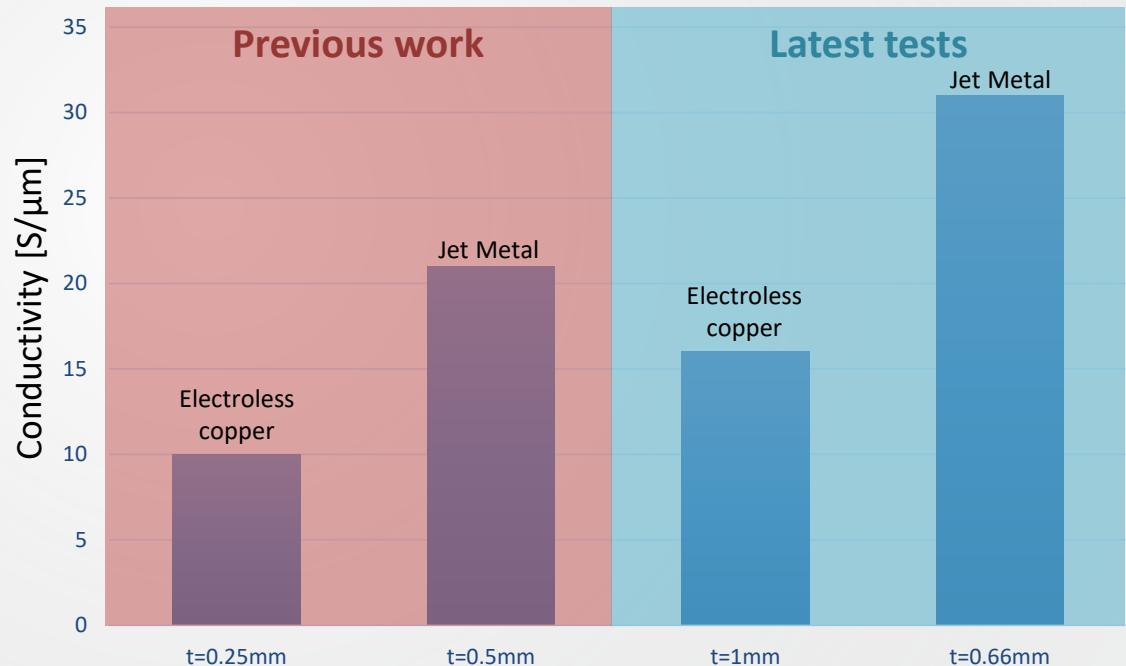
Metallization tests of Alumina substrates
