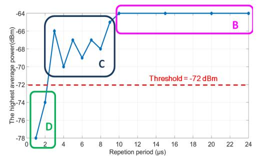
**B**: 10  $\mu$ s  $\leq$  T  $\leq$  24  $\mu$ s the *PHighestAvg* values are above the threshold of -72 dBm. Moreover, for these T values, the bit rate progressively decreases with the attenuation=Modulation and coding schemes (MCS) mechanism adjusts the bit rate to reduce errors caused by the interferences, until the power reaches the threshold for which the CCA-ED considers the medium busy.
