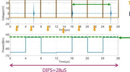
Time window for CCA calculation  $\leq 4\mu s = OFDM$  symbol + guard interval
