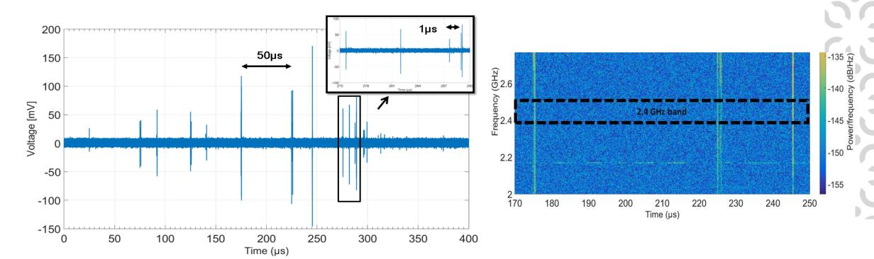
The transient EM interferences produced by the catenary-pantograph contact cover the Wi-Fi frequency band
