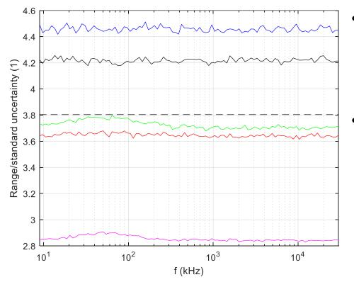
In the case of the triangular distribution the value of this ratio is  $2\sqrt{6}(1-\sqrt{0.05})$  and it is represented through a dashed line The triangular distribution is, in this sense, suitable to describe the spread of the possible values in the case represented by the green curve (i.e. when both z and k uniformly sample the borders of the corresponding domains)
