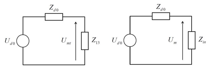
$U_{d0}$  is the open-circuit disturbance voltage generated by the EUT  $Z_{d0}$  is the EUT impedance
