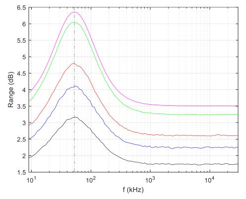
The range (difference maximum – minimum of the 95 % coverage interval) of  $\Delta$  is maximum at the frequency of 52,8 kHz, where the phase angle of the impedance of the 50  $\Omega$  | (50  $\mu$ H + 5  $\Omega$ ) AMN is maximum, whatever is the adopted sampling strategy
