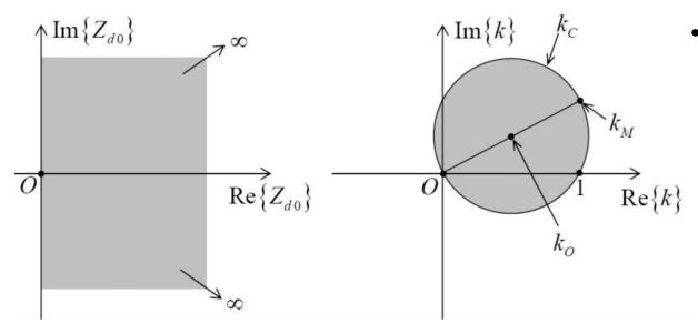
• Through the biunivocal transformation  $k = \frac{Z_{13}}{Z_{d0}+Z_{13}}$  the infinite domain of the impedance  $Z_{d0}$  (left) is transformed into the compact domain of the parameter k (right)
