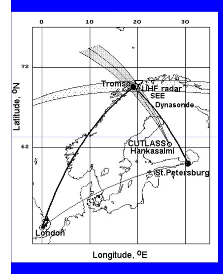
A map showing the experiment geometry. The EISCAT/Heating facility at Tromsø was used for HF ionospheric modification of the ionospheric F-region. HF heating facility was operating at at high heater frequencies ( $f_H = 5.423 - 7.953$  MHz) with the use of phased array 1 resulting in the effective radiated power of 450 - 650 MW.
