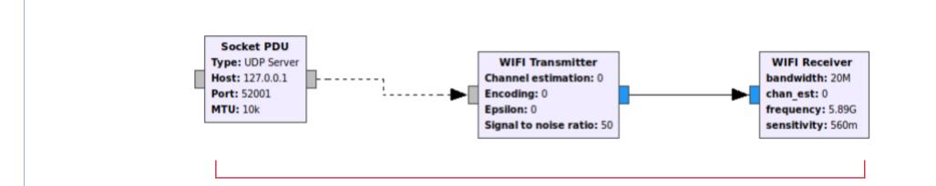
Wi-Fi beacons are transmitted periodically, as signals, by a Wi-Fi transmitter. They are received and decoded back into frames by a Wi-Fi receiver. The Wi-Fi receiver demodulates the signal and sent the frames to Wireshark [1] for frame analysis and calculations.
