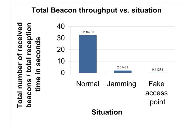
The number of lost beacons and the total beacon throughput confirms that in this experiment, the fake access point attack situation is the worst in beacon reception. A way to detect the fake access point on layer 2 of the OSI model would be to check if the beacon interval is the same at transmission and reception. In this case, the licit AP is emitting 1 beacon each 200ms (5 beacons per second) but the receiver has only received 0.11273 beacon in one second.
