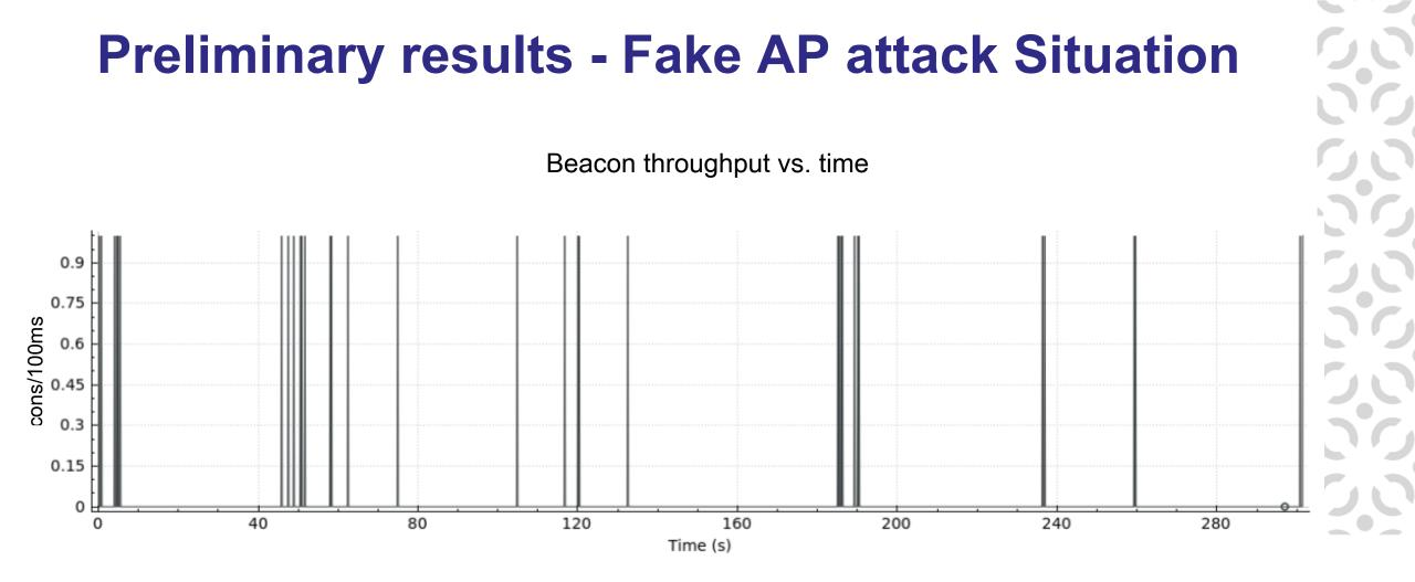
Here, we can clearly observe that at several instants, the beacons/100ms is zero. The reason can be due to the fact that the access points are emitting beacons on the same channel at a close interval of time (200 ms for the licit access point and 250ms for the fake access point), there is overlapping (interference) and the receiver can only decode beacons at instants where the interference is not so
