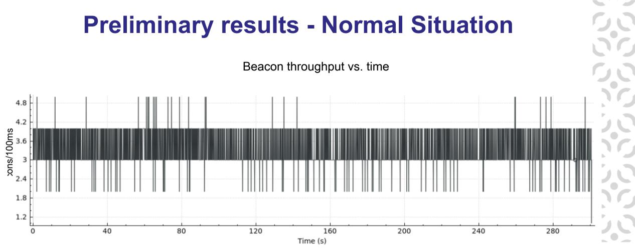
We observe that under the normal situation, the number of received beacons/100 ms is between 0.6 to 5 beacons/100 ms There are some fluctuations in the number of beacons/100 ms but the receiver received at least 0.6 beacon/100ms throughout the reception time. Provided that beacons are sent each 200 ms (0.5 beacon/100ms) and that packets cannot be lost under simulation, the amount of beacon loss for normal situation should be null.
