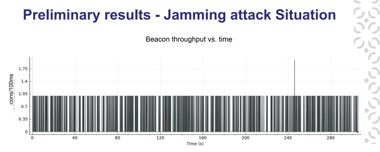
In contrary to the normal situation, we observe here that the number of beacons/100ms is within a smaller range and that there are several instants where the number of beacons/100ms is equal to zero. This indicates that the jamming had an effect on the reception and has led to the loss of beacons and more generally performance degradation.
