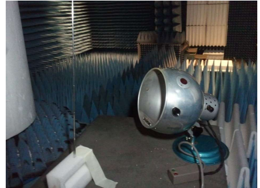
Fig.-2: Measurement arrangement inside an anechoic chamber
