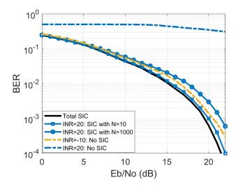
**Figure 2.** Comparison of the BER performance of the FDSM system with different SIC levels (total SIC, no SIC, SIC with 10 or 1000 test numbers)
