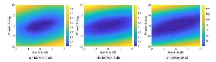
Figure 3. Relative BER of the FDSM system in presence of IQ imbalance under Eb/No=10,15 and 20 dB
