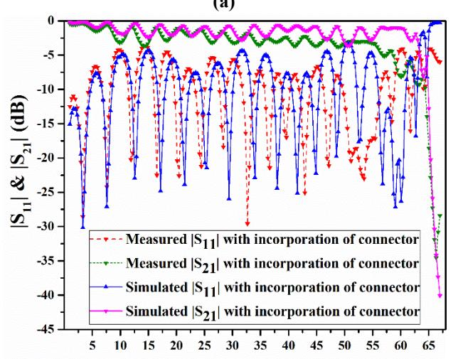
**Figure 4.** (a) Fabricated prototype of the proposed transmission line structure, (b) Magnitude of the simulated and measured reflection  $|S_{11}|$  and transmission coefficient  $|S_{21}|$ . [inset: size of the developed transmission line].
