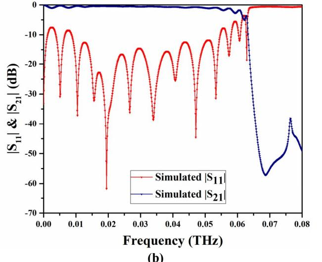
**Figure 3.** (a) Schematic of the proposed transmission line structure, (b) Magnitude of the simulated reflection  $|S_{11}|$  and transmission coefficient  $|S_{21}|$ .
