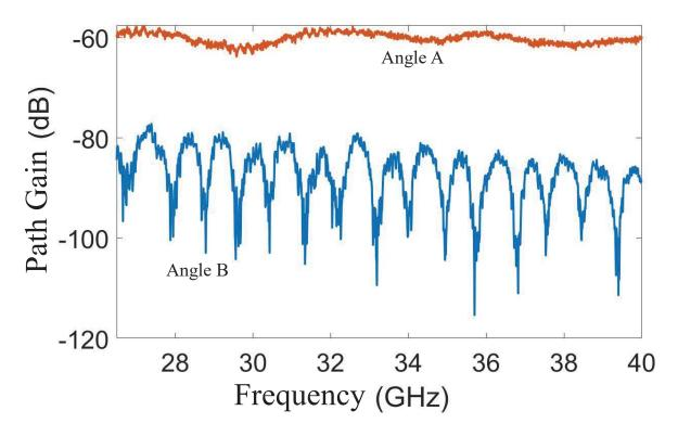
Figure 3: The high multipath propagation channel path gain frequency response provided for the metal tank (Angle A) and bank of control boxes (Angle B).
