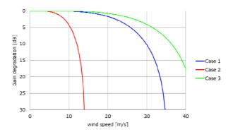
**Figure 6:** Wind speed vs. Gain degradation for three cases of pole thickness and pole hight
