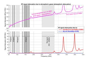
**Figure 2.** Frequency-dependent RF signal attenuation due to atmospheric gases (atmospheric attenuation), and as a reference, total propagation loss (free space loss + atmospheric attenuation) at a distance of 100 m.
