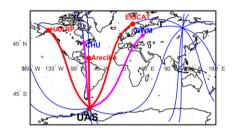
**Figure 1**. Map of the experiment. It is shown the direct (red for heaters and magenta for time and frequency service) and opposite (blue) radio paths. The length of direct radio paths to UAS from: HAARP – 15600 km, CHU – 12300 km, Arecibo – 9200 km, EISCAT – 16300 km, RWM – 15100 km.
