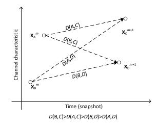
**Figure 1.** Illustration of different trajectories between the MPCs.  $\mathbf{x}_i^m$  and  $\mathbf{x}_i^{m+1}$  are the MPCs in *m*-th snapshot and m + 1-th snapshot, respectively, whereas  $D_i$  is the distance between different MPCs.
