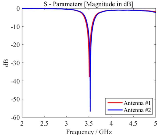
**Figure 5.**  $S_{11}$  results for the Antennas #1 and #2.
