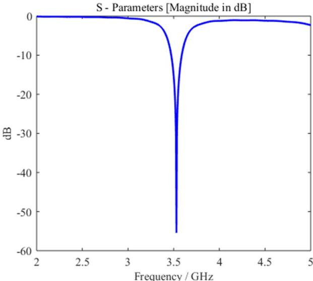
**Figure 7.** S<sub>11</sub> results for the Antenna #4.
