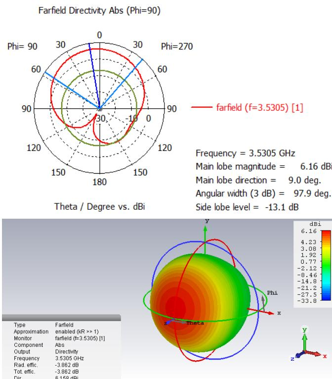
**Figure 8.** Far field pattern results for the Antenna #4.
