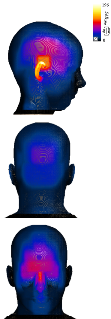
Figure 2. Distribution of SAR_{10g} induced by the 8x8 planar array antenna at 3.7 GHz for 100 mW input power on the head skin model. In the upper part for the lateral configuration, in the middle part for the posterior one and in the lower part for the frontal one.
