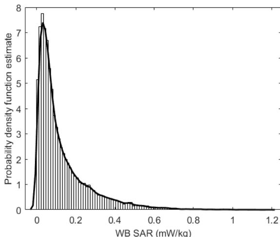
**Figure 2.** Histograms and probability density function of the WB SAR values for 100.000 random positions of the WLAN source and the child.
