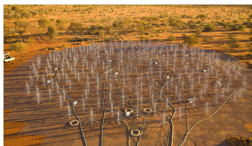
Figure 1. An aerial side view of the AAVS2 array, November 2019. Credits: ICRAR/INAF.
