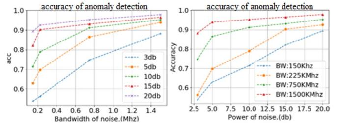
**Figure 5.** Accuracy of anomaly detection for the pulse interference with different power and width.
