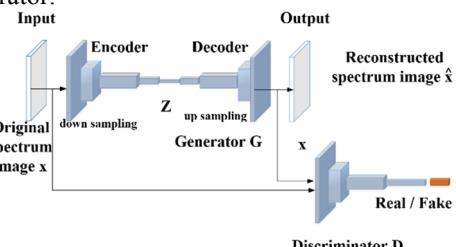
**Figure 1.** Structure of improved GAN model
