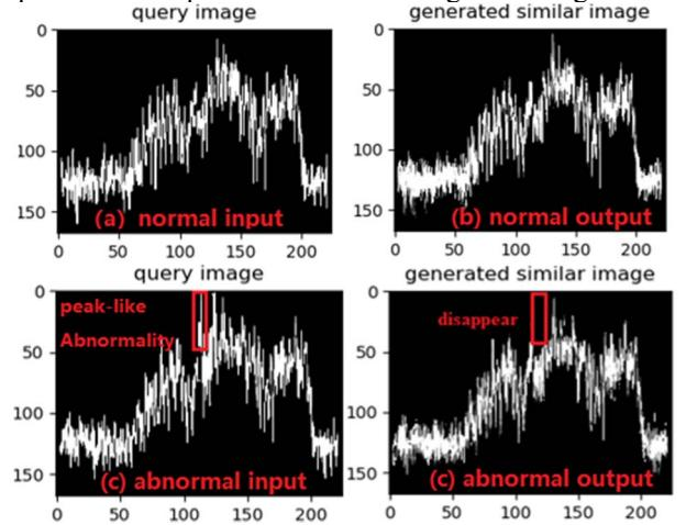
**Figure 4.** Process of detection for both normal and abnormal spectrum images
