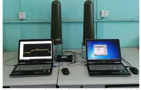
**Figure 3.** Receiver (left) and transmitter (right)
