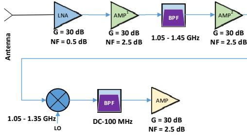
**Figure 2.** A single frontend signal path framework and the parameter design.
