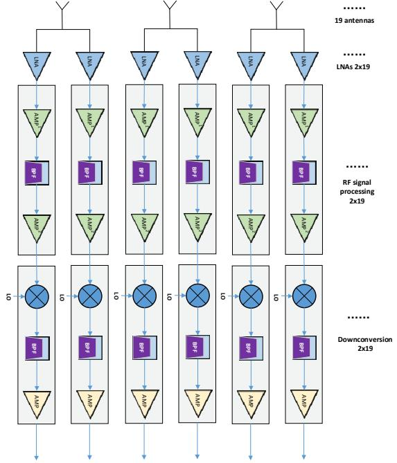
**Figure 3.** 19-element PAF frontend signal paths framework.
