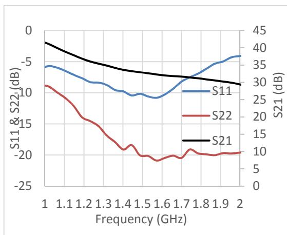
(b) S-parameter measurement results of the LNA
