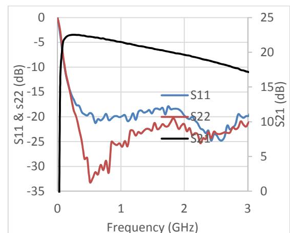
(b) S-parameter measurement results of the RF amplifier
