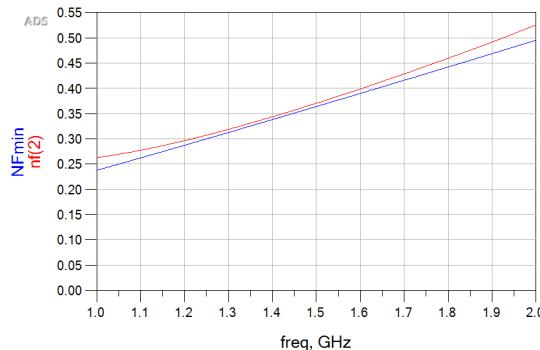
**Figure 4.** The noise performance simulation of the LNA.
