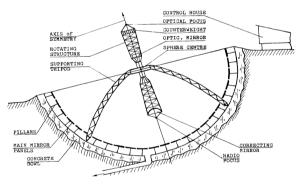
Figure 1. Arrangement of Radio-Optical Telescope ROT-54/2.6.
