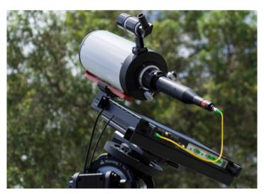
Figure 1. Optical terminal for the free-space phase-stabilized frequency transfer system.
