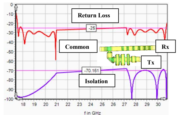
Fig. 4. Diplexer return loss and isolation performance
