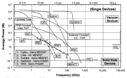
Fig. 3.2.1 Average RF output power versus frequency for various electronic devices<sup>11</sup> and semiconductors.<sup>12</sup>
