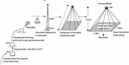
Fig. 2.4.13 Overall construction scenario
