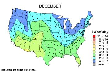
Fig. 2.1.3 Minimum insolation by two-axis tracking flat plate<sup>6</sup>
