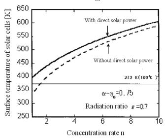
Fig. 2.3.7 Sun light concentration rate and balance temperature of generator ( $\alpha$  absorption ratio of solar power;  $\eta_G$ , efficiency of solar cell)<sup>32</sup>
