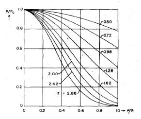
Fig. 3.1.2 (Right) Relative cross-section power density distribution across the transmitting and receiving antenna apertures for various values of  $\tau$  as given in Fig. 3.1.1. R is the radius of the transmitting or collecting antenna and  $\rho$  is the radial distance from the center. The field at the collector extends beyond its edges. <sup>1,3</sup>
