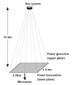
Fig. 2.4.11 1GW class Tethered-SPS
