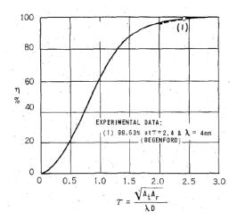
Fig. 3.1.1 (Left) Transmission efficiency as a function of parameter  $\tau$  for optimum power density distribution across the transmitting antenna aperture as shown in Fig. 3.1.21<sup>1,3</sup>
