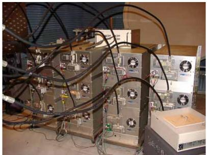
Fig.2.3.11 Phased Array with 12 Phase Controlled Magnetrons at 2.45 GHz © RISH, Kyoto University
