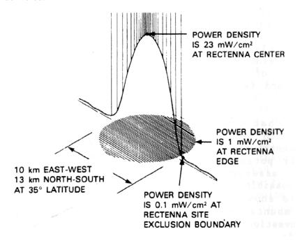
Fig. 2.4.3 Power density distribution at rectenna site on the ground.
