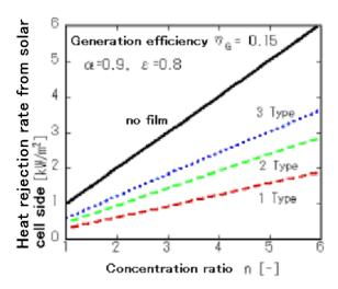
Figure 2.3.10 Relation between sunlight concentration ratio and heat rejection rate (with spectral filter attached)<sup>33</sup>
