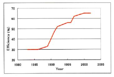
Fig.2.3.12 Trend of Efficiency of TWTA<sup>45</sup>
