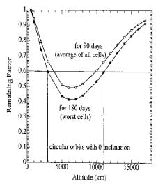
Fig. 2.3.2 Deterioration of efficiency of the solar cells during 6 months Altitude vs. Remaining Factor -
