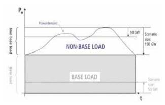
Fig. 2.4.15 Definition of base- and peak-load (non-baseload) power as used for the present assessment.
