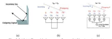
Fig. 2.3.15 (a) Two-sided corner reflector (b) Van Atta Array (c) phase-conjugating array. (Sung et al., http://hcac.hawaii.edu/tcwct03/papers/s16p03.pdf)<sup>56</sup>
