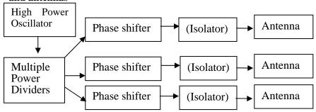
Fig. 2.3.13 Implementation of microwave transmission with a high power microwave oscillator and phase-shifters for high precision control of microwave beam direction to large angles without grating lobes<sup>37</sup>
