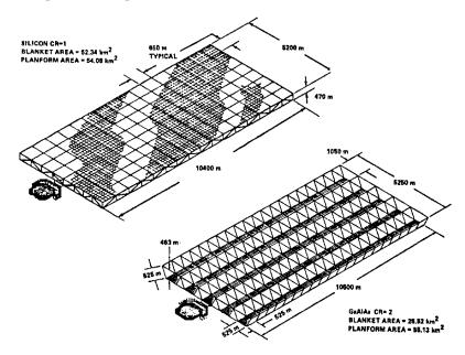
Fig. 2.4.2 NASA-DOE SPS Reference Model
