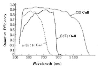
Fig. 2.3.9 Spectral sensitivities of solar cells<sup>35</sup>
