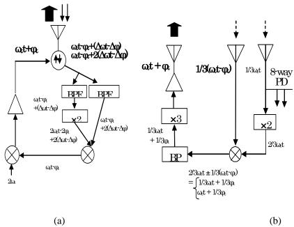
Fig. 2.3.16 Phase conjugate circuit developed in Kyoto University © RISH, Kyoto University
