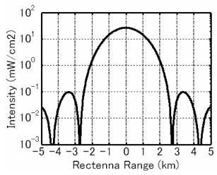
Fig. 2.2.1 Typical power density at a rectenna site (1kmφ TX antenna with 10dB Gaussian power distribution)
