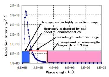
Figure 2.3.8 Effects of a spectral filter set between the sun and the solar cell<sup>34</sup>
