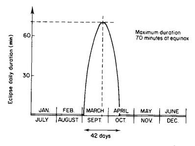
Fig. 2.1.2 Daily duration of eclipses as a function of the date.<sup>2</sup>
