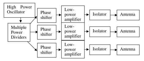
Fig. 2.3.14 Implementation of microwave transmission with phase shifters and low-power amplifiers for high-precision control of microwave beam direction without grating lobes<sup>37</sup>
